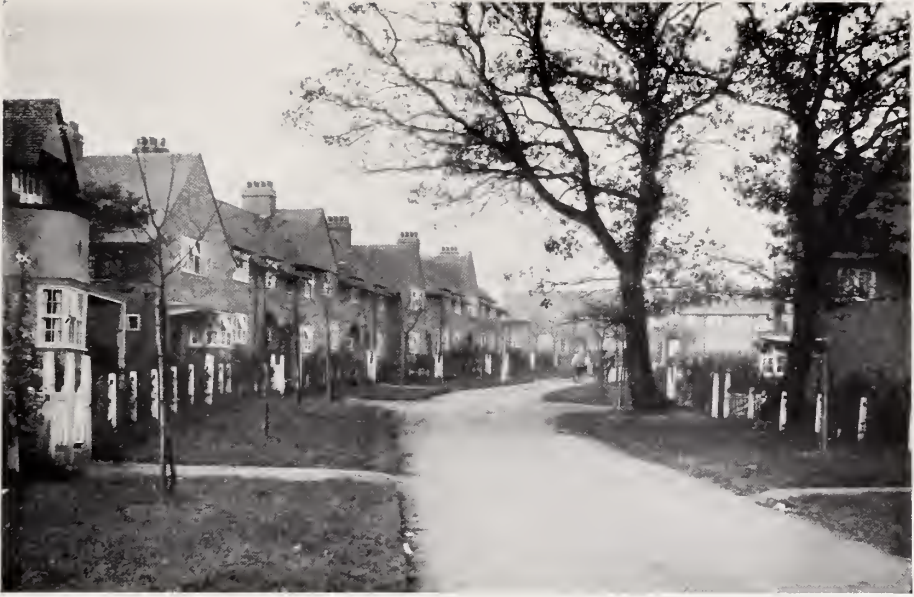
Illus. 227.—Asmunds Place, Hampstead Garden Suburb. A carriage drive used in place of an expensive road. Photo by Mr. J. P. Steele, Stoke-upon-Trent.
